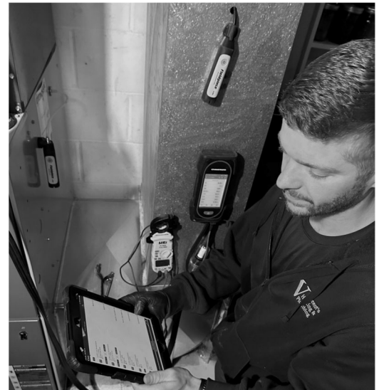
Here is Nathan inside the house with more mQ probes attached to the furnace ductwork looking at a live measureQuick analysis on his iPad.
